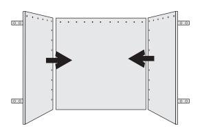
Lay the box on its back and attach the top making sure the flanges are facing upwards and then secure in place.
