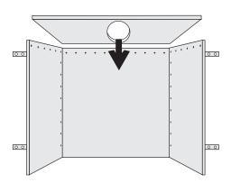
When all the joints are tight, silicon inside the box and clean off which makes a seal at all the joints. Leave to dry. DO NOT FIX THE COLLAR AT THIS POINT.
